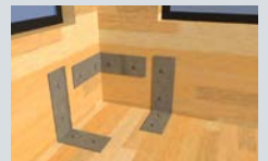
Panels are fastened simply with large brackets and bolts, making assembly easy
